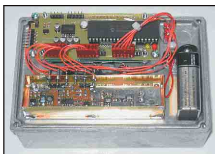
Fig 5—Inside view of the meter. The CPU module is on the top, the RF measurement section is on the bottom. The LCD is mounted under the CPU module.
